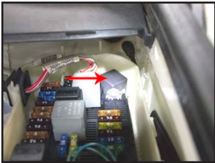
02-09 Mercedes-Benz E-Class Relay located on the left side of the vehicle by the firewall.
