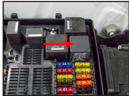
04-10 Jaguar XJ Series Relay located on the right side of the vehicle in the engine compartment.
