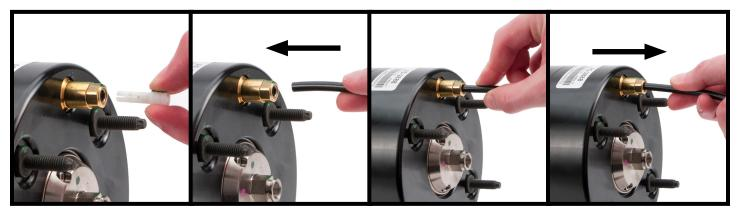
REMOVE AND DISPOSE OF THE SHIPPING PIN.
