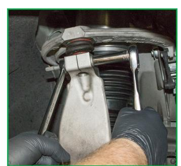
5. Reinstall the sensor wire bracket and reattach the end link to the lower strut clevis. (Figures 28, 29, 30)
